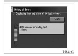
7. If trouble items are displayed with time count, repair/replace the system according to "ERROR HISTORY" TABLE, EL-410.
